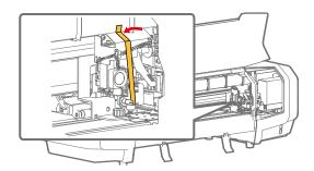
Secure the sheet cutter with tape.
