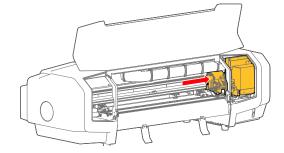
Manually move the carriage to the platen where you can easily install the blade holder.
