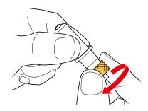
Calculate the blade depth using the calculation formula of target blade depth (thickness of film + thickness of backing material)
