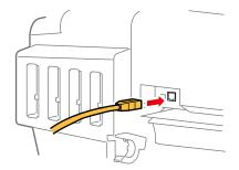
Secure the Ethernet cable with the cable tie.
