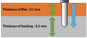
Use the above as a guide when making an adjustment.
