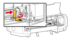
Secure the contour cutter with tape.
