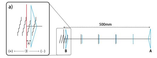
Example b) If the width of the pattern is set to 500 mm and the cut line was off from the reference line by eight vertical lines of the scale lines to the non-origin side:
